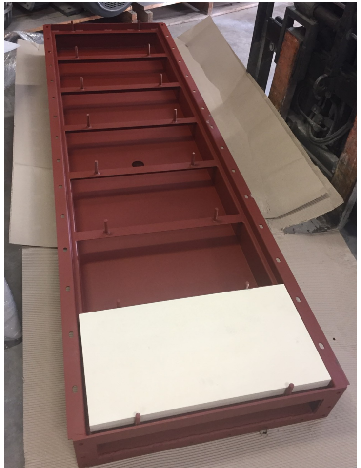
New porous ceramic tiles being installed into the steel frame.
