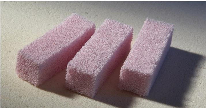
**Puremet** is a unique ceramic formed as a reticulated irregular, three dimensional, open cell structure with a high average surface area. It is ideal as a catalyst, bio-mass support medium, or metal pour filter for the casting industry.
