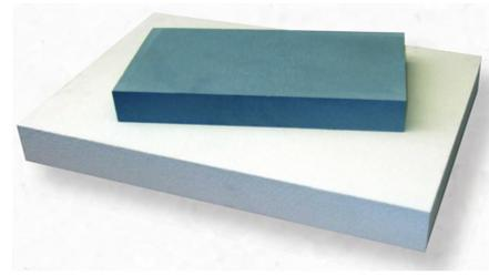
Porous ceramic tiles are subject to close control during manufacture. Individual tiles are matched one against the other to ensure even overall permeability and the grades used present sufficient resistance to spread the air evenly over the whole area.
