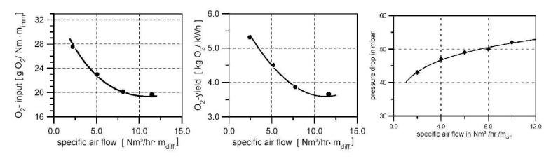
Measurements were taken under standard conditions according ATV M209 (clean water, water depth = 4,0 m, average density of aerators 0,9—1,2 m<sub>diff</sub> / m2)
