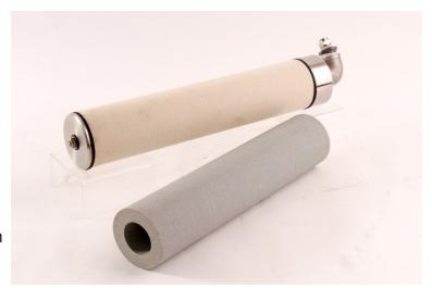
The ceramic diffuser tubes are typically mounted on the distribution pipe with centering bosses and end caps by means of a tie rod with. The aeration piping is installed at the bottom of the aeration tank. Depending on the material chosen for the piping, the ceramic tube diffusers are fastened to the piping either directly or by means of tees.
