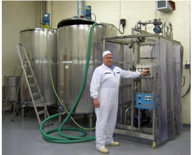
Ransom's Crossflow Microfiltration System incorporating Mantec's Star-Sep™ Ceramic Membranes
