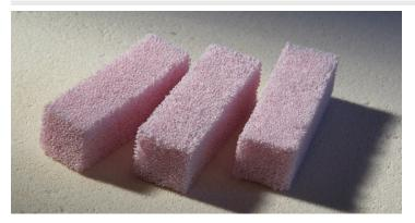
**Puremet** is a unique ceramic formed as a reticulated irregular, three dimensional, open cell structure with a high average surface area. It is ideal as a catalyst, bio-mass support medium, or metal pour filter for the casting industry.
