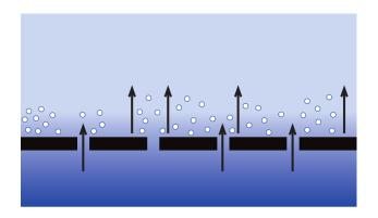
Also, the air is mixed with the material in such a way that the friction between the particles is reduced, allowing the material to flow like water.
