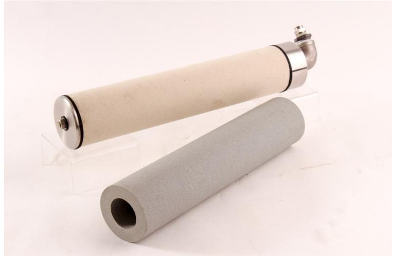
The ceramic diffuser tubes are typically mounted on the distribution pipe with centering bosses and end caps by means of a tie rod with. The aeration piping is installed at the bottom of the aeration tank. Depending on the material chosen for the piping, the ceramic tube diffusers are fastened to the piping either directly or by means of tees.
